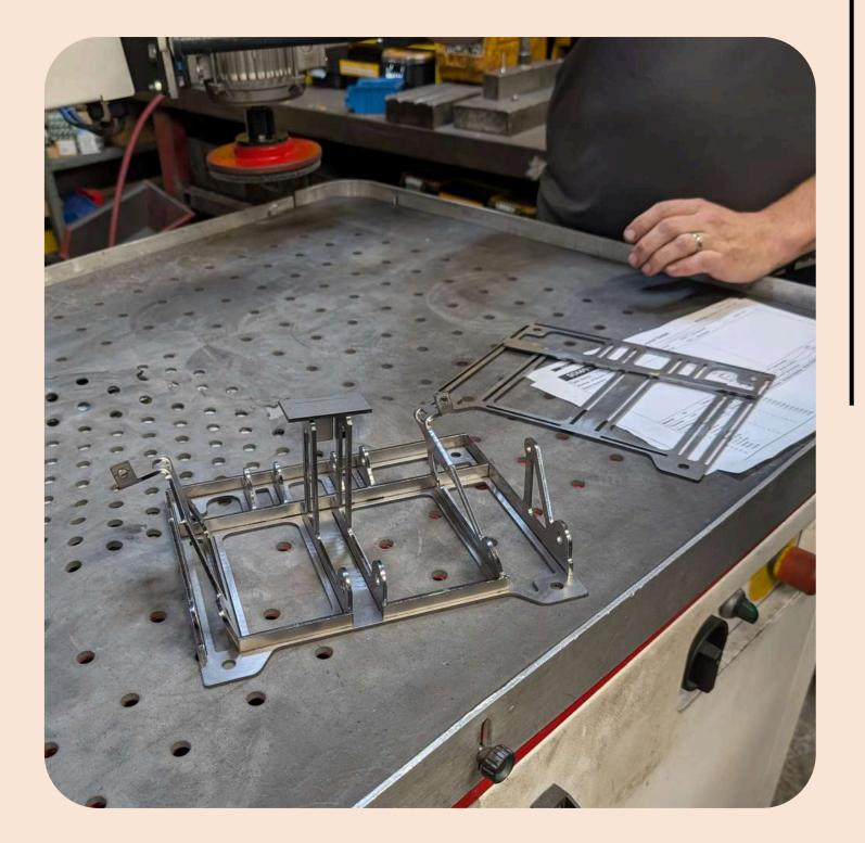
Development of a new radiator package is underway with the initial design undergoing validation before it progresses for its design review at PMA Automotive Cooling. This will be a crucial step towards understanding the final design constraints for both the radiator packaging itself and the sidepods.
