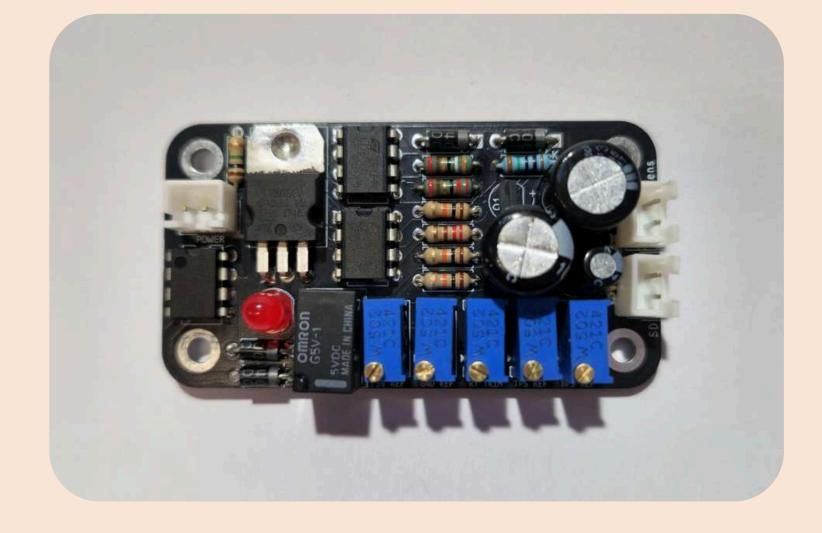
The team has also completed the manufacture and testing of the Brake System Plausibility Device (BSPD) this device is part of the safety system and will shut the car down when both the throttle pedal and the brake pedal are pressed (seen above). This is a really important component as it is required in the regulations. Having this component completed this early in the year allows for ample time for the Controls sub-team to test this component thoroughly for bugs and reliability.
